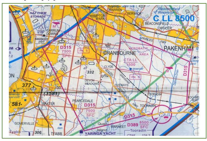
D315 is a Danger Area, from Surface to 7500 feet and is specified as Flying Training. West of us is the Aerobatic Area signified by the red box which should be the area used for engine out manoeuvres.
