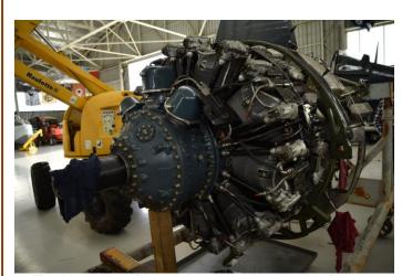
The big beast of a radial engine, thousands of Horse power, note the massive prop' shaft
