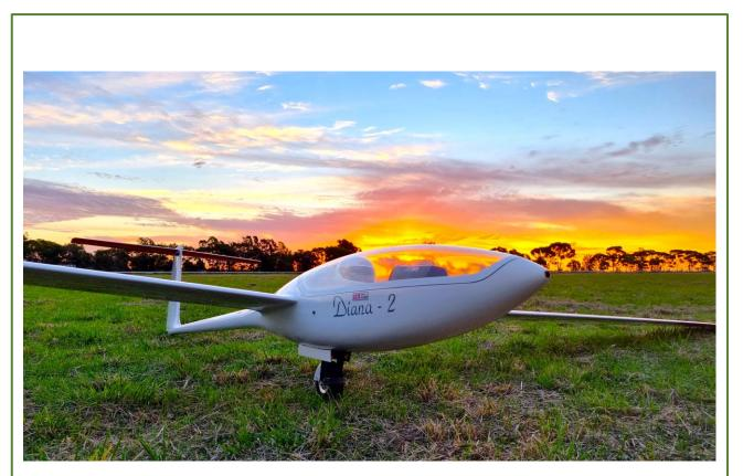
Keith Quiggs' Diana 2 scale sailplane by Baudis Models in the Czech Republic. At 1/3 scale it has a 5.5 metre wingspan, weighs in at 9kg depending on ballast used. Full composite construction.
