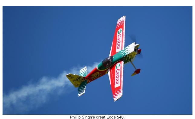
50% scale, wingspan 3.7M, ARF with balsa and ply construction, Flying weight 27kg, up front is a 375cc petrol engine, running a 37 X 14 prop', the colour scheme follows the full size plane owned by Pip Borman, an Australian Aerobatic flyer who tragically lost his life, when his Pitts Samson he was flying crashed near Shepparton Airport in 2009
