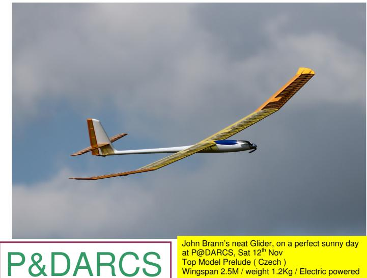
Top Model Prelude (Czech) Wingspan 2.5M / weight 1.2Kg / Electric powered
