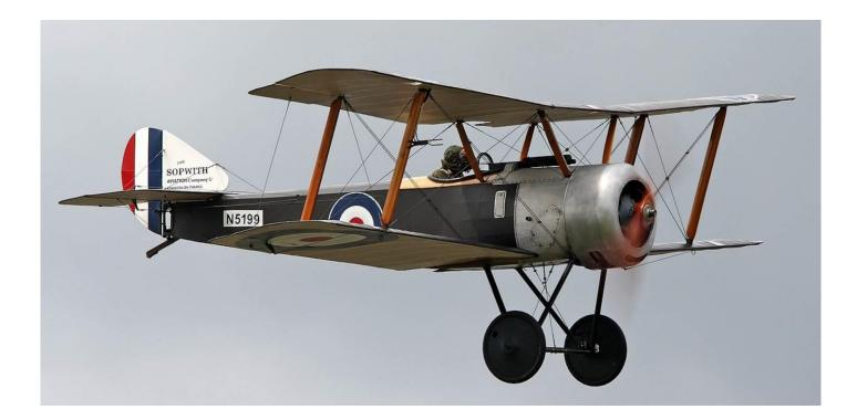
While some aircraft still used wing warping the Pup not only used ailerons but had them on both wings. This feature along with a very light wing loading and careful rigging made this aircraft comparatively easy to fly. A modern day pilot coping with a rotary engine, where the *entire engine rotated* with the propeller might beg to differ.
