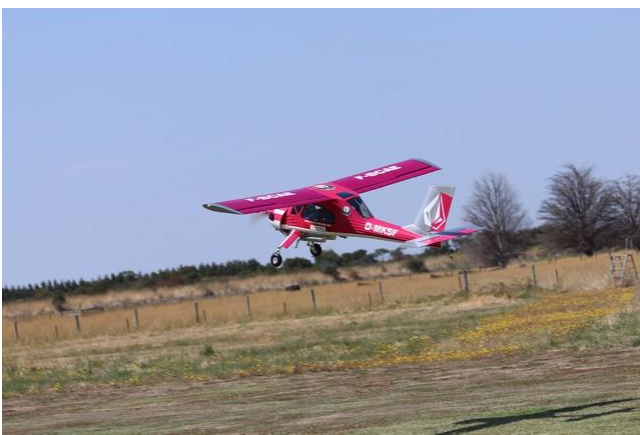
Michael Lui's Wilga lifting off, Wilka PZL104, 3M span, DLA 112cc twin petrol, set up for glider aero tow
