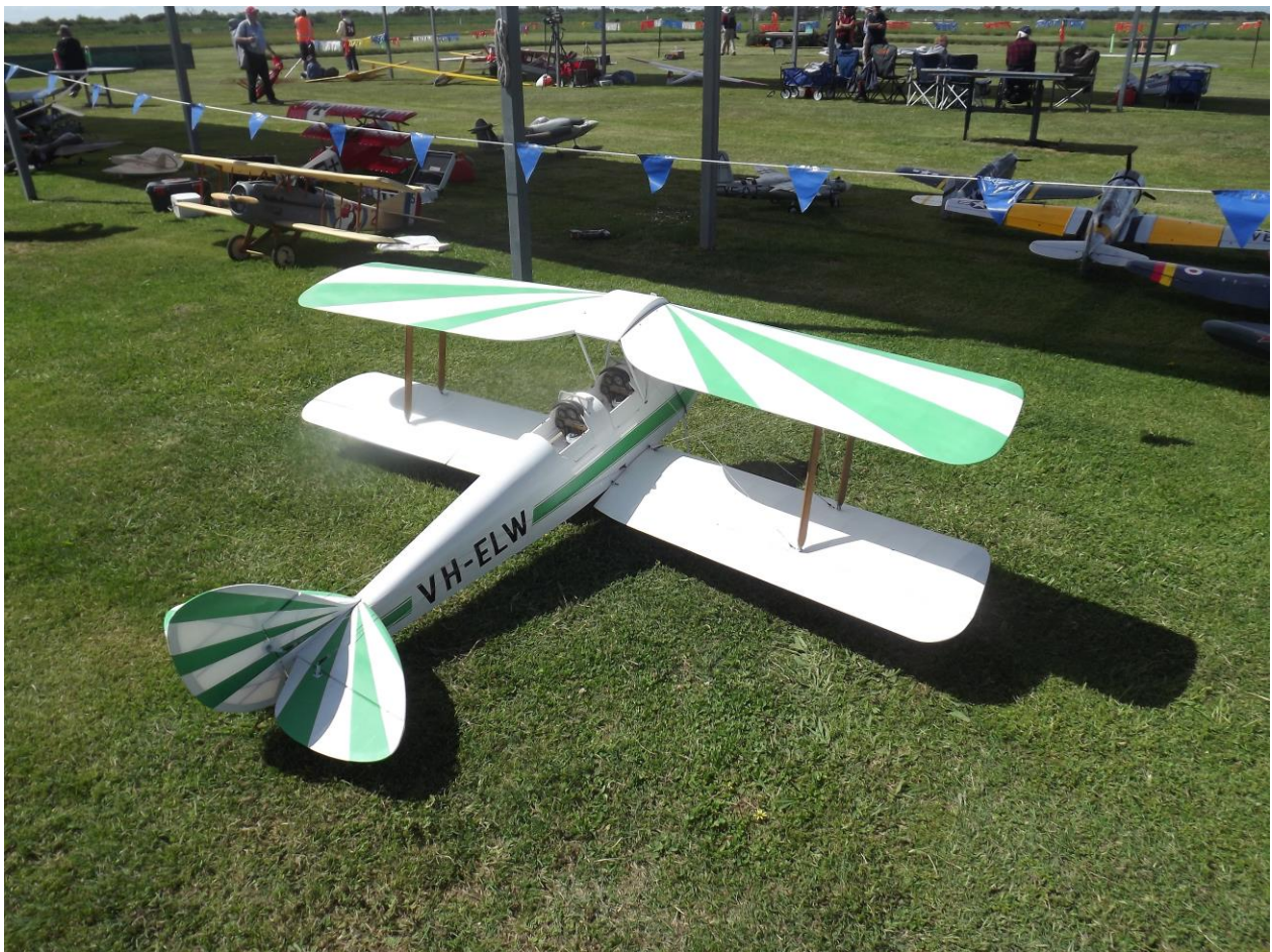
Don White's nice \frac{1}{4} scale ( 84 inch ) Pilot Kit, Tiger Moth, O.S 129 F/S with diaphragm pump, all up weight 7 Kg, Don is yet to have it certified, Photo taken at 2019 Monty Tyrell
