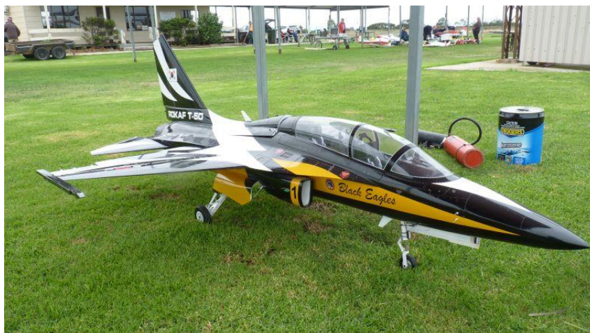
Dave Law's Black Eagles jet, Rokaf T50, Swi Win 190 turbine, 90Kg thrust, wet weight about 18Kg, span about 1.7 M, from Dragon R.C
