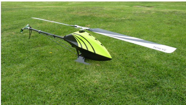
Hung Tran's custom made Heli', made in Suzi, Laos 800 size, electric motor quantum 45 300, 500KV, ESC 160 amp, Futaba flybarless controller
