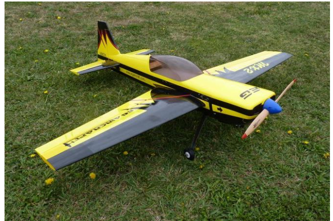
Hung Tran's MX2, 3D, balsa and ply, DLE 30cc petrol, 1.7M span, 18 x10 prop
