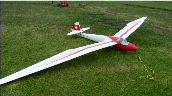
Tim Morgan's ¼ scale Mimi Moa pre WW2 German glider, span about 5.2M, ARF from Dragon R.C
