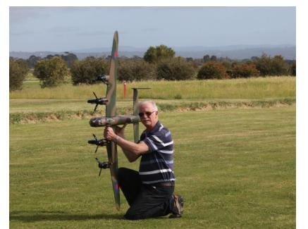
Alan Foley with his nice scratch built 72" Lancaster, 4 electric SK3 1040Kv, swinging 9 x 6, 3 blade master airscrew props' motors controlled alternate in pairs, from two Lithium Batteries, the scale is, 14:1, built from plan by Tony Nijhuis, Laser cut ribs and formers by Andrew Smallridge, covered in 1.5mm balsa, with sikspan and 8 coats of dope, the paint finish was airbrushed
