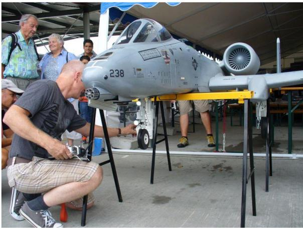
Adjusting Brake on Nosewheel
