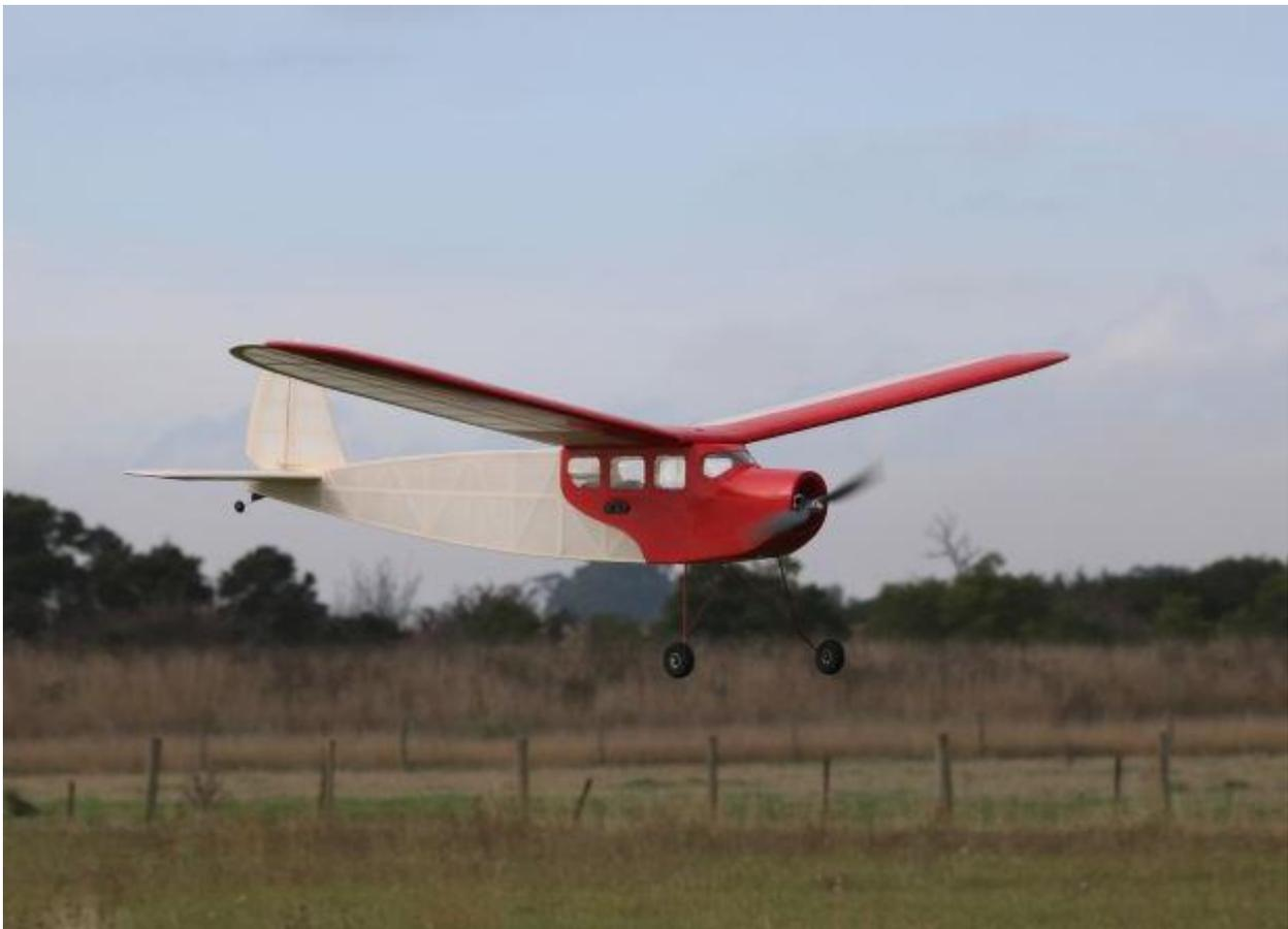
Geoff Healey's nice 1936 Miss America, 84 inch span, electric powered, covered in original Silkspan and dope, at our field, on 15<sup>th</sup> May this year
