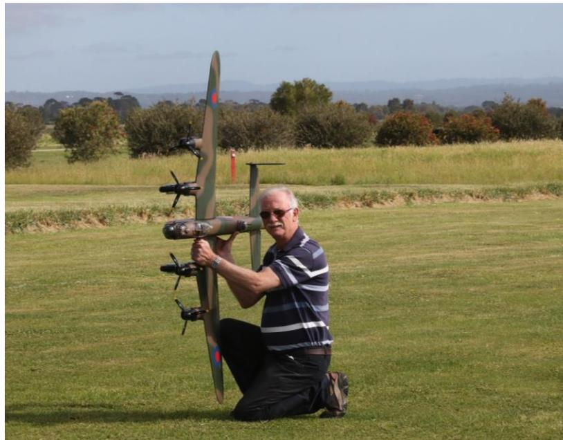
Alan Foley with his nice scratch built 72" Lancaster, 4 electric SK3 1040Kv, swinging 9 x 6, 3 blade master airscrew props' motors controlled alternate in pairs, from two Lithium Batteries, the scale is, 14:1, built from plan by Tony Nijhuis, Laser cut ribs and formers by Andrew Smallridge, covered in 1.5mm balsa, with sikspan and 8 coats of dope, the paint finish was airbrushed
