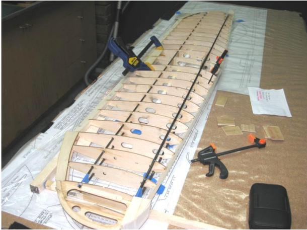
Wing building on the plan, note the carbon fiber spars
