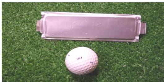
A typical LiPO ( pouch ) cell, 5 amp hours, beside a golf ball to judge size, The small tabs on the ends are the + and - electrical connections
