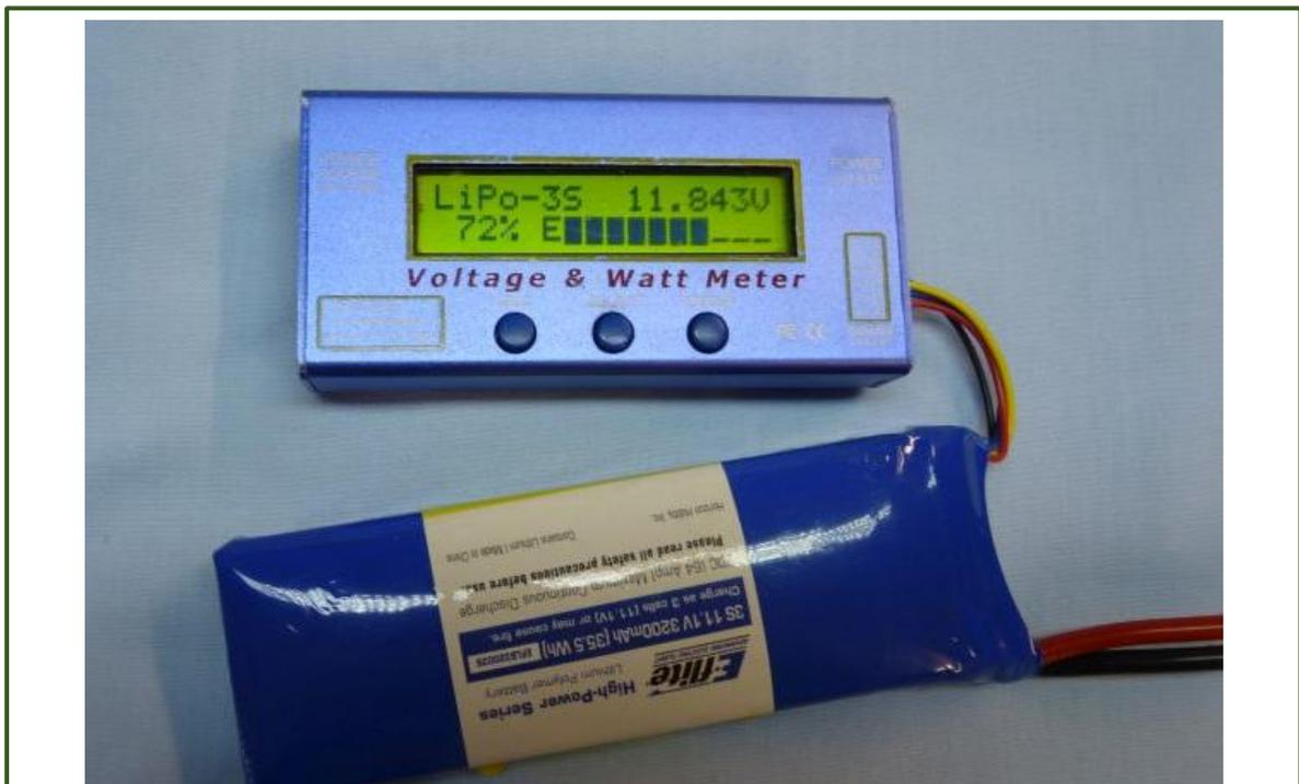
A typical battery tester, set to test a LiPO, the display shows, it is set for LiPO, 3 cells ( 3S )
