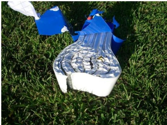
An impact damaged 6s 5000mAh LiPO pack
