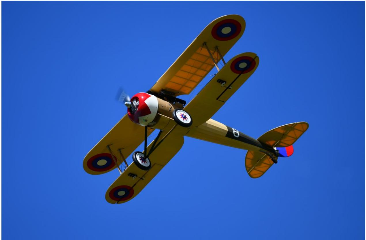
Owner/builder Bruce Clarke's lovely Nieuport Biplane. Build from the Balsa USA 1/6 scale kit, has a 1.2 metre wingspan, flying weight, around 3.5kg, covering is Solartex and finished with Humbrol paints. Power comes from a Magnum 52 four stroke, and guided by the Spektrum DX9 radio system.
