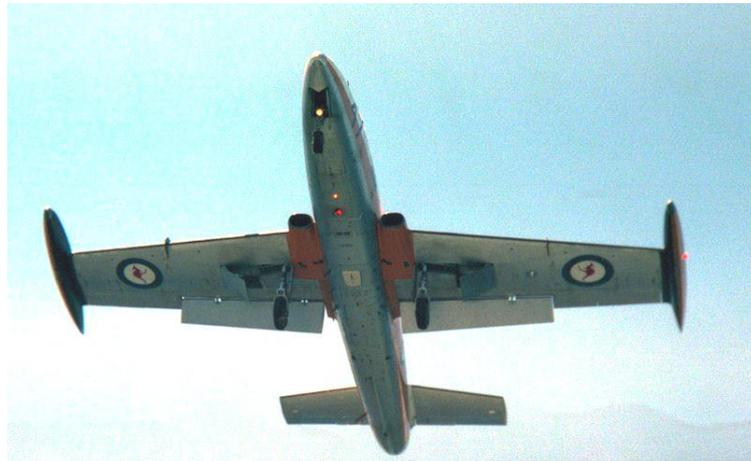
An RAAF Macchi MB-326, off Fremantle during a flypast of Australian aircraft carrier HMAS Melbourne, circa August 1980 ( note the wing flaps deployed )
