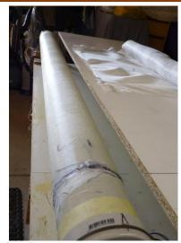
The first fiberglass pressure chamber on a water pipe mandrel, waiting for the epoxy to set, it is around 1500mm long
