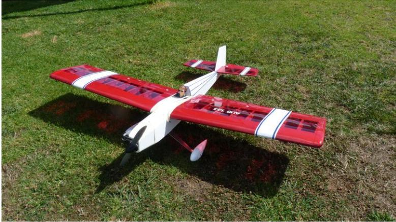
Cliff McIvor's Fun Fly Sportster, scratch build during lockdown, flaps, 120 O.S 4 stroke pumped, loads of power
