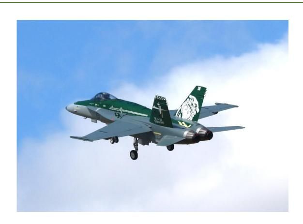
Dave' Chivers fabulous FA-18 Hornet climbing out, on it's maiden flight on Monday 3<sup>rd</sup> January BVM Models U.S.A , 1 : 5.5 scale, Wingspan : 2.2M, Length : 3M, Power : 2 off Kingtech K320 turbines, for 32Kg thrust, Weight : about 25Kg including 6L of fuel, ( jet A1 )
