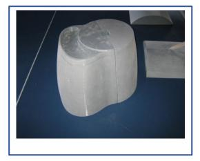
They used a 3 view to make a 3D software model using 3D software which Andrew is very good at manipulating. He then "cut" it up into sections and then is in the process of 3D printing them with Ivan putting them all together to create the plastic "plug". Ivan is doing the wing design on normal CAD which will be covered with G10 when built.
