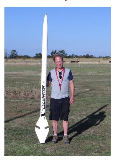
Rick' (Rockets) Talman, at our Flying Field early 2017, with his big X-celerator, Solid fuel rocket,100mm diameter, parachute recovery, easily capable of achieving 4,000 feet +
