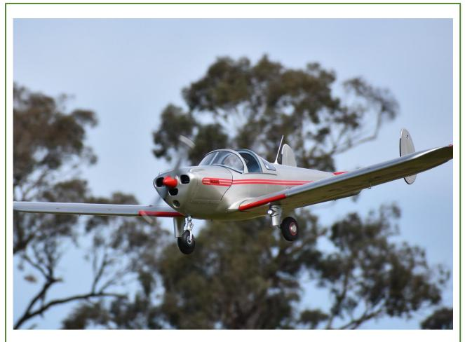
This nice Ercoupe from Tim Dehann was built from a 1/3 scale Balsa USA kit. Tim added many scale details to the basic kit and has modelled it on a full size Ercoupe which is based at Tyabb Airport. Power is via a Saito FG-61TS four stroke petrol engine, and the radio system is a Spektrum DX18. As you can see from the photo, Tim has done an outstanding job on the model.
