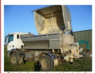
Reloading lime spreader truck from hydraulic dog trailer hopper
