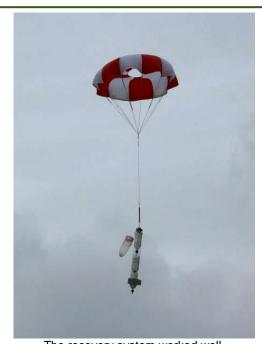
The recovery system worked well, Later, the chute got saturated with rain water, it got chucked out o.k but it didn't open
