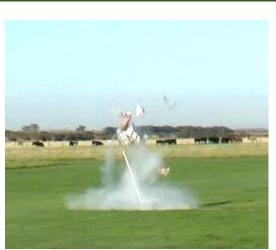
Failure of the coupling between container 1 and container 2, the white fog is the 2 liters of water in container 1 vaporized, the launch rail was set at that angle
