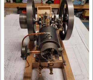
Rick Talman's very well made Red Wing model engine, it is 4 stroke, with a centrifugal speed control, that opens the exhaust valve, on a Hit & Miss basis
