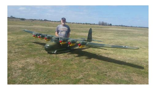
Mark Collins with his 1/12<sup>th</sup> scale ME323, 4.2M wingspan / 24kg / 6 off 46LA motors, a long ground run to get airborne, at the field for certification by Neil Addicott from Model engines The Messerschmitt Me 323 *Gigant* ("Giant") was a German military transport aircraft of World War II.
