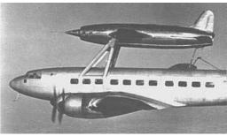
The Leduc aircraft qualify as a strange aircraft not only because of the radical power plant but also because of the extraordinary fuselage configuration. The air intake circled the entire fuselage and the cockpit had to be positioned in what looked like a spike coming out of the engine. This severely limited cockpit space and indeed the pilot did fly it from a lying
