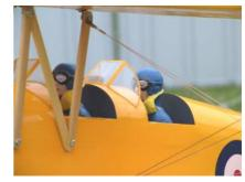
had a lot of negative incidence. To overcome this I had to shorten the rear inter plane struts. I made some new ones, as there would not be enough meat on the originals to drill new mounting holes. Holes were drilled in the fuselage and the cabane struts screwed to the fuselage. The wings are mounted!
