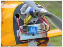
The model is designed to be flown with a 40 - 46 noise. I had no intension of going down this path. My son, Stephen, offered a 30mm Hyperion outrunner motor (HP Z3025 - 8) to power the model. I accepted. With a 45 amp ESC and 3S2P LiPo battery of  $8000 \, \text{mA}$  capacity the model would fly very similar to the prototype.
