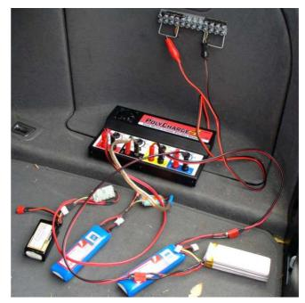
My only minor beef with the unit is the inbuilt fan runs continuously even when not charging, which leads to the possibility you might flatten your car battery if you leave it connected for a long period without using the car. That detail aside, I highly recommend the charger to anyone who likes to keep a plane and fully charged batteries in the boot for whenever the wind is light and you pass a nice park....
