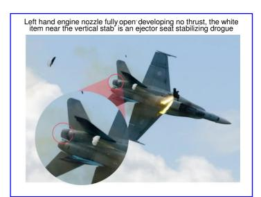
Notice the pilot's head pinned to his chest from the severe "g" forces produced by the solid rocket motors in the ACES II seat. They burn for about 2/10ths of a second, enough time to propel him at least 60 feet clear of the aircraft, ejected canopy at the rear
