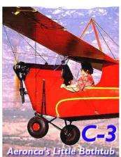
The fuselage was quite bulky as it needed to be wrapped around the aforementioned pilot and as the engine was mounted so high and the propeller was so tiny there was no need for a long undercarriage and indeed it looks like it was connected directly to the fuselage. That must have resulted in an atrocious ride over rough ground or on less than perfect landings.
