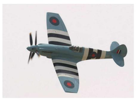
Up to five propeller blades were needed to absorb the power of the Griffon and in one of the greatest visible changes to a Spitfire some variants were fitted with two contra rotating three bladed propellers!
