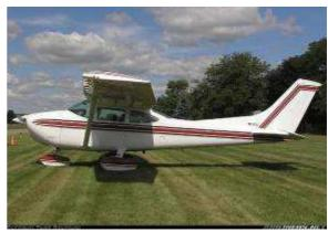
make the Cessna range look more modern by raking the fin and rudder and cutting down the rear fuselage to accommodate a rear window. The raked fin and rudder were of course less effective, although not as much as perhaps imagined, and the airflow around the rear window was obviously going to be a source of increased drag....and who was going to be looking out of that rear window anyway?
