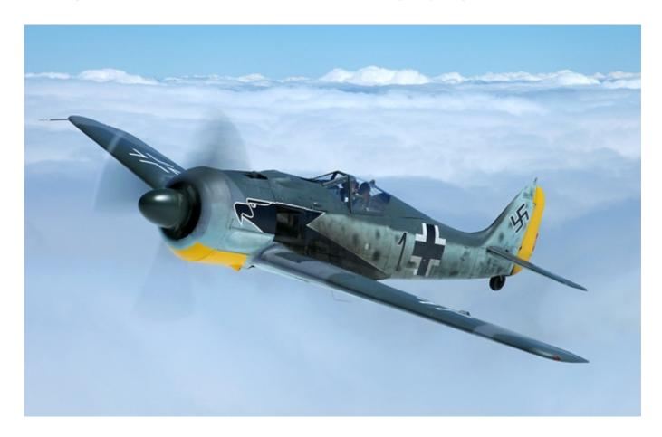
A lack of turning ability was due to the relatively small wing. That small wingspan however led to more speed and greater maneuverability. Its pilots loved it, finding it much easier to fly than that other great Luftwaffe fighter, the Me 109. In particular the wide undercarriage made landing much easier. An extraordinary number of Me 109s were lost in landing accidents.
