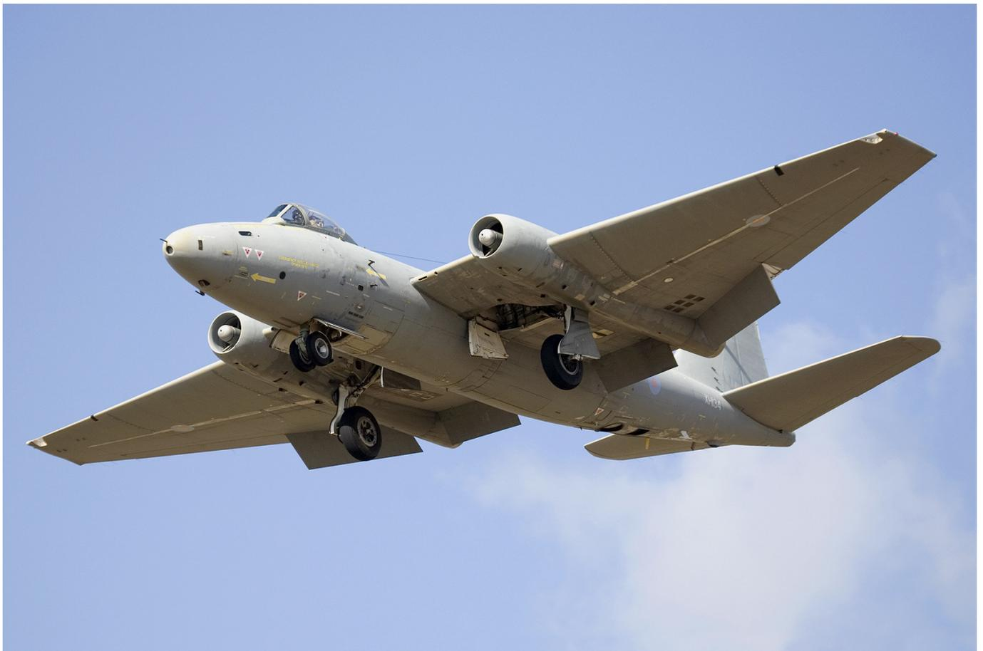
An early semi aerobatic display at the Farnborough Air show met with official disapproval! There was an early problem with rudder over balance which was cured by slicing the top off the gracefully curved fin and rudder resulting in the unusually squat looking vertical tail.
