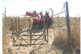
The forklift tine unit being used to lift and tow a scrap frame from the windmill / dam area
