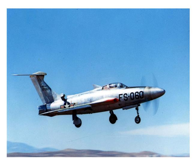
XF-84H "Thunderscreech" was based on the F-84F Thunderstreak but was fitted with a turbo prop on the front and retained its normal jet engine in the back. The Turbo prop had a supersonic propeller. Its name, Thunderscreech, is a reference to its extremely loud supersonic propeller which made it the loudest plane ever made.
