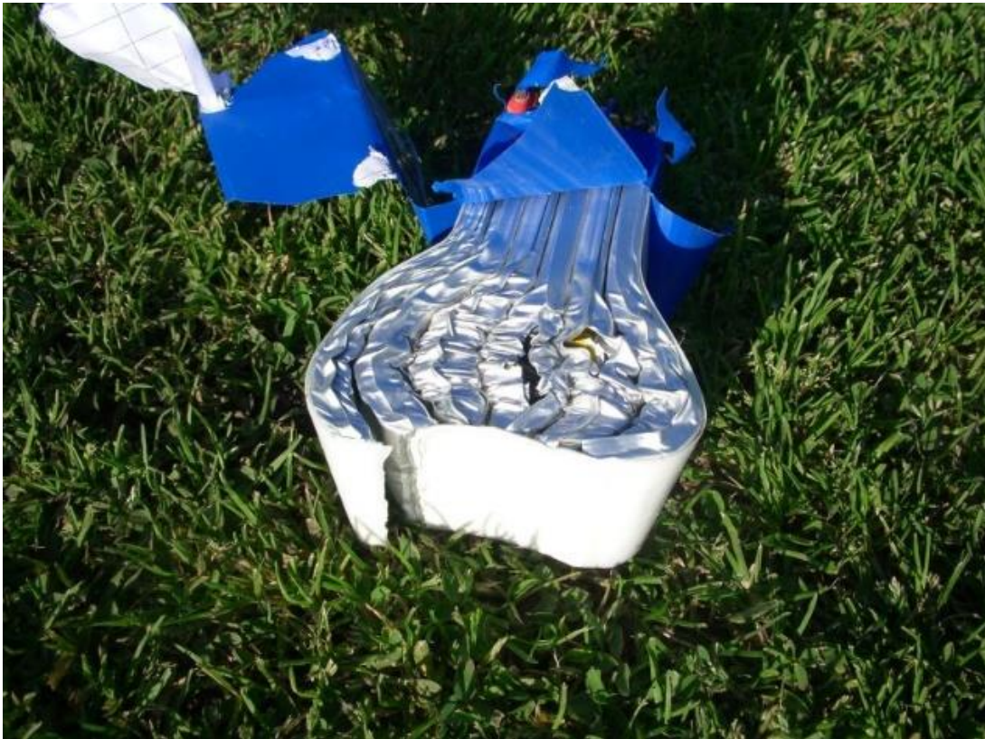
An impact damaged 6s 5000mAh LiPO pack, ( it did not burn ! )
