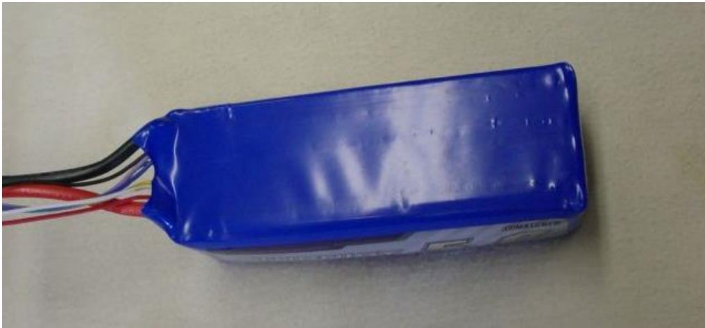
A badly swollen 6s 5000 mA hr LiPO pack, very risky to continue using this one
