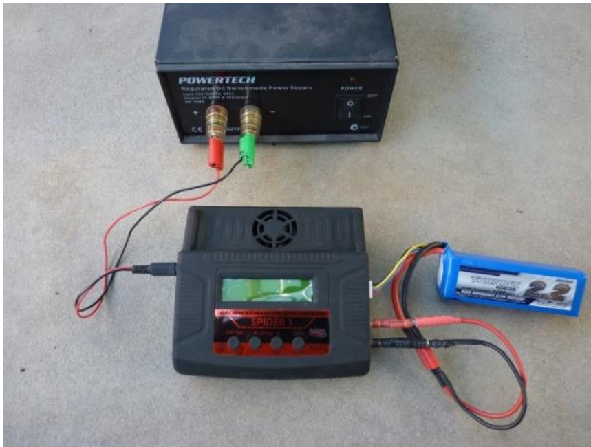
A typical computer-controlled charger, and power supply, on a concrete surface
