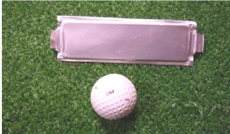
A typical LiPo RC ( pouch ) battery pack, 5000mAh, beside a golf ball to judge size The small tabs on each end are the + and - electrical connections
