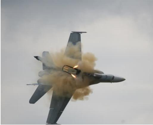
Left hand engine nozzle fully open developing no thrust, the white item near the vertical stab' is an ejector seat stabilizing drogue
