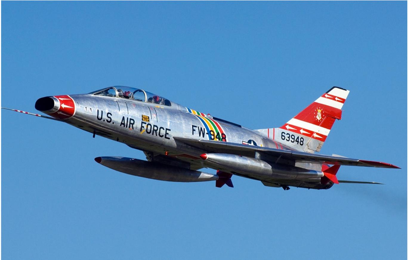
The Super Sabre was the first of the renowned " Century Fighters ", the aircraft designated F-100 to F-105 culminating in the late sixties with the General Dynamics F-111, a swing – wing two-seater that carried eight tons of bombs and rockets at 1650 mph.
