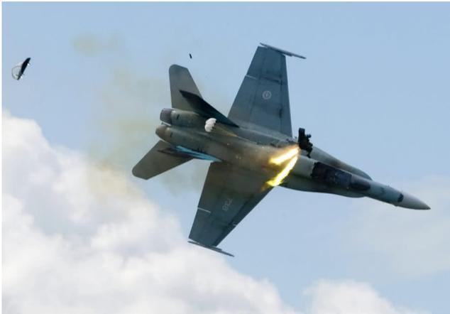
Close to impact, the chute' is still slowing the pilot, the seat following the aircraft down
