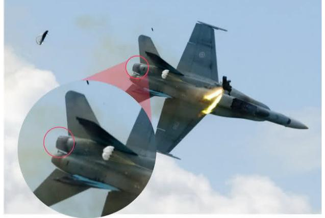
Notice the pilot's head pinned to his chest from the severe "g" forces produced by the solid rocket motors in the ACES II seat. They burn for about 2/10ths of a second, enough time to propel him at least 60 feet clear of the aircraft, ejected canopy at the rear
