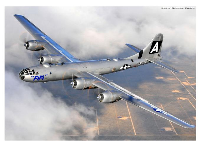
A major advance was that it was to be pressurized which avoided the crippling cold and oxygen mask breathing which the B-17 and Lancaster crews had endured at bombing heights.
