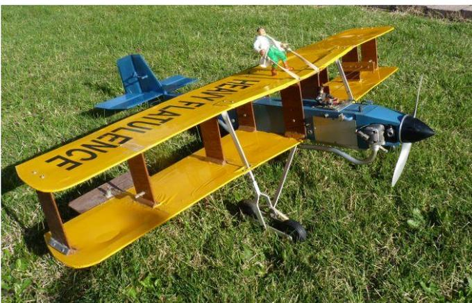
An unusual model, called " Heavy Flatulence " **Heavy**, as the whole thing is made from 3 ply, **Flat** as the wings have a flat profile, the **Uulence** refers to the motor exhaust piped to the rear of the model, O.S 46 LA power, plus many other unusual features, should be fun
