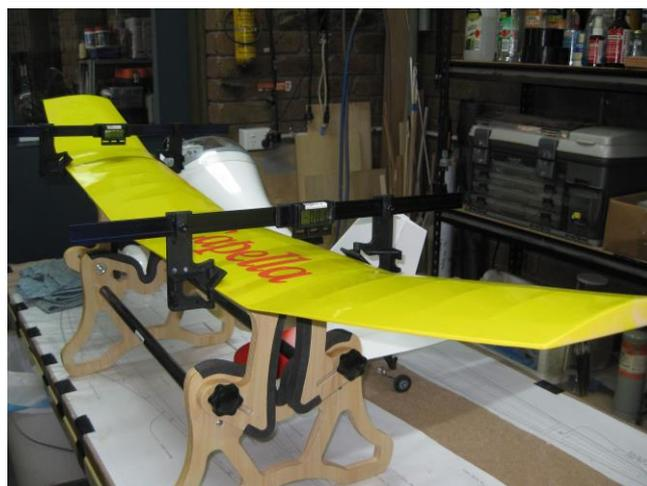
The wing tested true on the incidence meters
