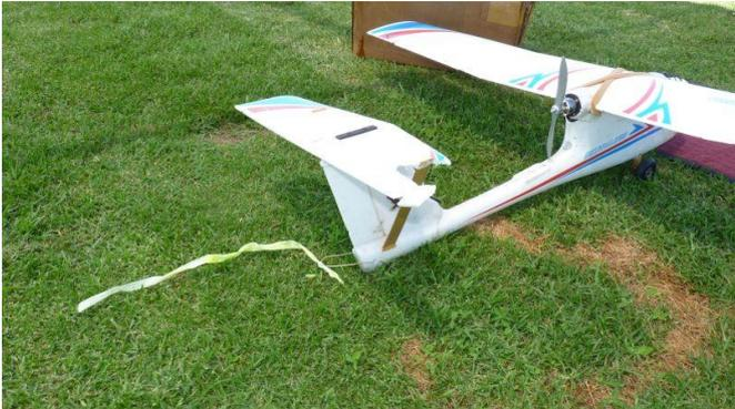
Frank McPherson's streamer towing foamy model after having a hunk of the elevator chopped off during a mid-air
