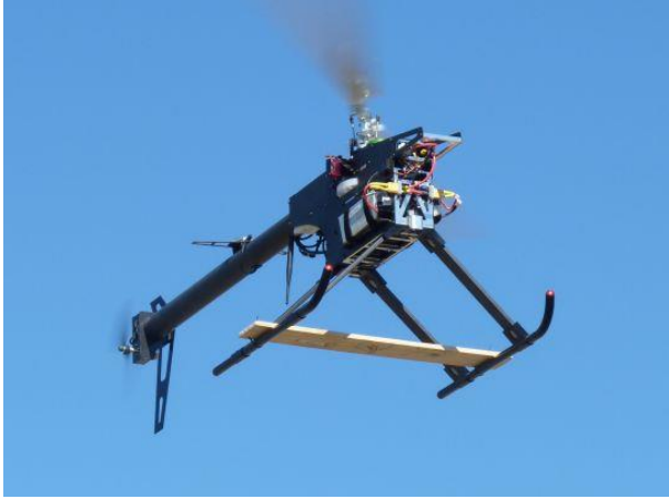
Steven Greig's large commercial UAV Helicopter The machine is used for Power line inspection / land survey, single 2M rotor, can carry a max' 10KG load, uses a 12S 16,000mAh LiPO battery, and is equipped with ballistic recovery
