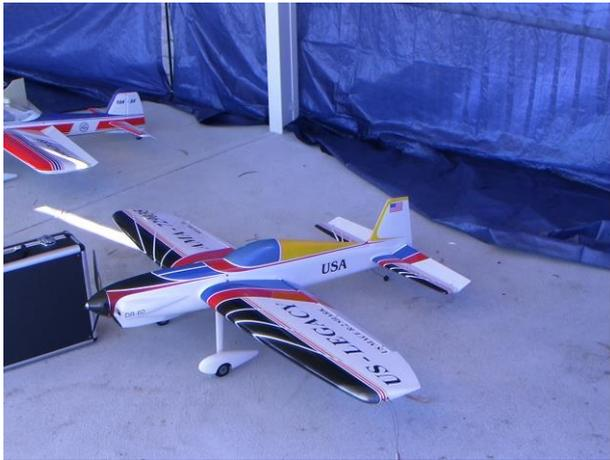
Aerobatic models, half of them now electric power, with automatic speed controller for constant speed during vertical maneuvers
