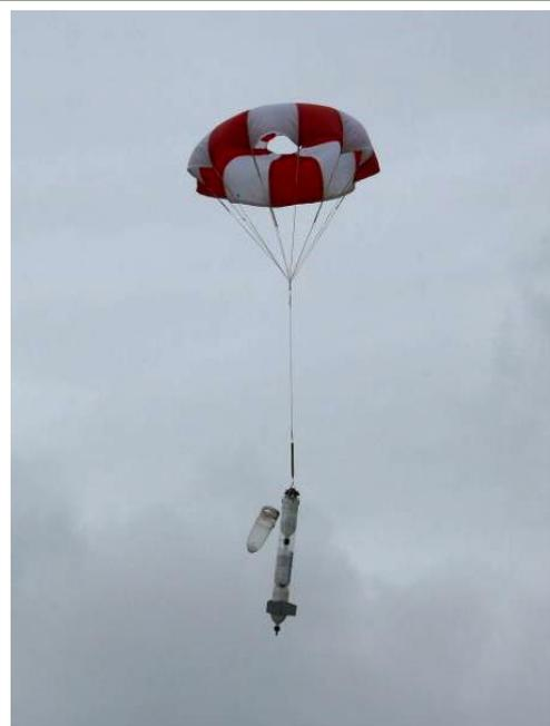
The recovery system worked well, Later, the chute got saturated with rain water, it got chucked out o.k but it didn't open
