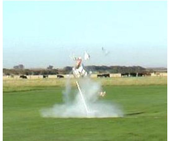
Failure of the coupling between container 1 and container 2, the white fog is the 2 liters of water in container 1 vaporized, the launch rail was set at that angle
