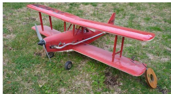
Little red biplane, model of a 1940s " Currie Wot "46 LA, extended exhaust, control lines storage roll sitting on inside wing
