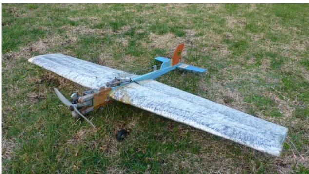
This is a control line trainer, called a UKI, it has a foam wing, elevator control only, 46 LA power, stick fuselage, all ready to go
