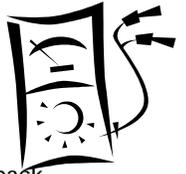
To test total current draw, connect the meter between the receiver and battery pack.
