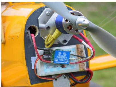
The model is designed to be flown with a 40 - 46 noise. I had no intension of going down this path. My son, Stephen, offered a 30mm Hyperion outrunner motor (HP Z3025 - 8) to power the model. I accepted. With a 45 amp ESC and 3S2P LiPo battery of 8000mA capacity the model would fly very similar to the prototype.
