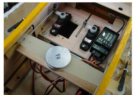
to a servo. The wires are connected to the bar with kwik links connected to 2/56 threaded wire. Nylon covered stranded wire loop at the rudder through 1/2A control horns. Not completely scale - but looks good.
