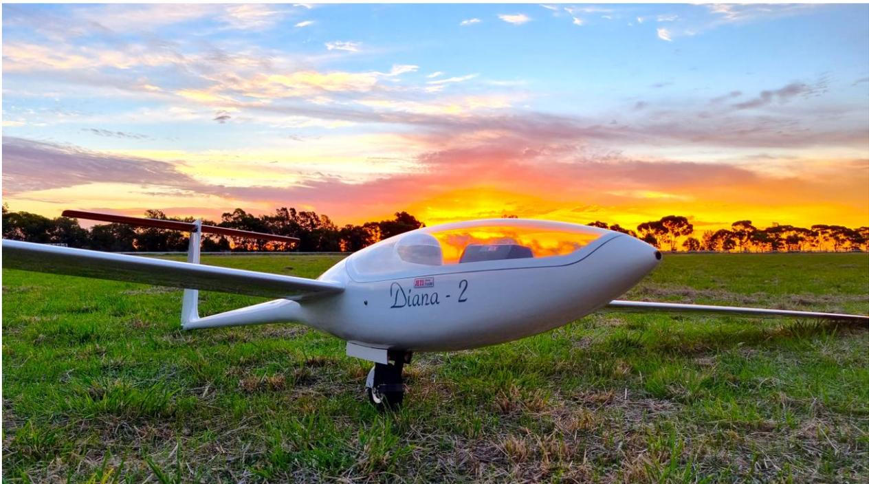
Keith Quiggs' Diana 2 scale sailplane by Baudis Models in the Czech Republic. At 1/3 scale it has a 5.5 metre wingspan, weighs in at 9kg depending on ballast used. Full composite construction.
