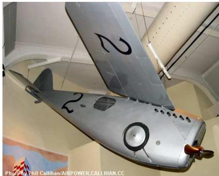
The aircraft had a variable camber wing in that the leading edge could be drooped in conjunction with the trailing edge flaps for slow flight. This was automatically done as the undercarriage was lowered for landing. *Undercarriage lowered?* I hear you ask. Yes, this was one of the very first aircraft to have a reliable method of raising and lowering the undercarriage. Not only that but to combine that action with variable camber wing was not often seen again until the F-16 etc!
